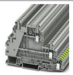
Ground modular terminal block, Connection method: Screw connection, Cross section: 0.14 mm² - 6 mm², AWG: 26 - 10, Width: 6.2 mm, Height: 60.1 mm, Color: gray, Mounting type: NS 35/7,5, NS 35/15
